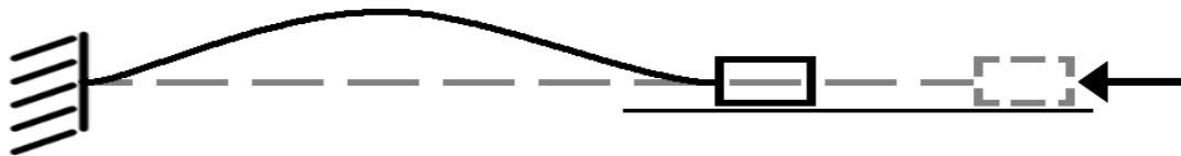
Figure 3.3 Linear beam buckled under a compressive load
